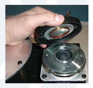
The diaphragm and plate adapter are easily removed from the horn assembly. They may not be broken down any further. Place the new diaphragm (part # coming soon) and plate assembly where the old one was. Follow the same steps as above, but backwards 4 to 1. Power up the SA1530z and the new diaphragm should now be pumping out those highs again. Sweet, you just replaced a diaphragm!
